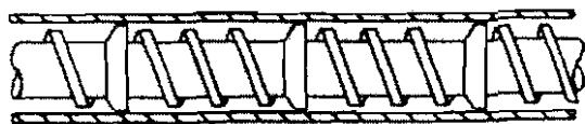
CONSTANT ROOT DIAMETER, CONSTANT PITCH SCREW WITH RESTRICTIONS IN CONSTANT DIAMETER BARREL
