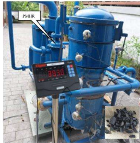
Fig. 4. Charcoal consumption rate measurement.
