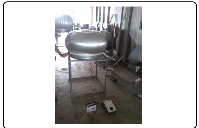
Fig. 14. Generator testing with roof ventilator
