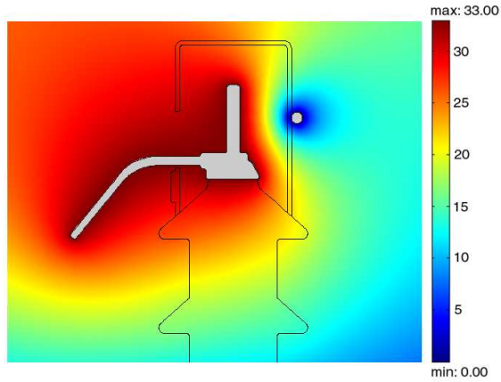
Fig. 9. Voltage distribution around porcelain bushing and bushing insulator when bushing insulator contacted with grounding tree branch.
