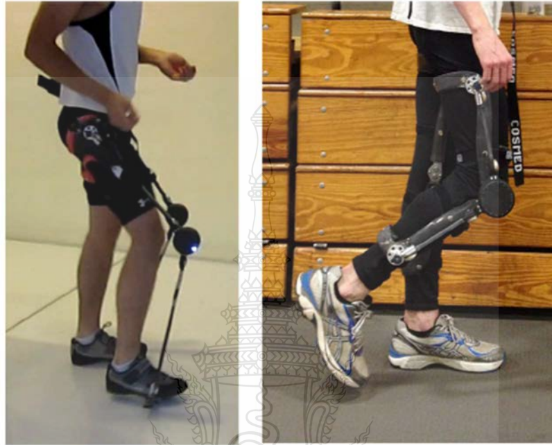
Figure 2. 4 Clutch Spring Knee Exoskeleton for Running (SOURCE: Design of a clutch-spring knee exoskeleton for running. Journal of Medical Devices, Transactions of the ASME, 8(3), 2014)
