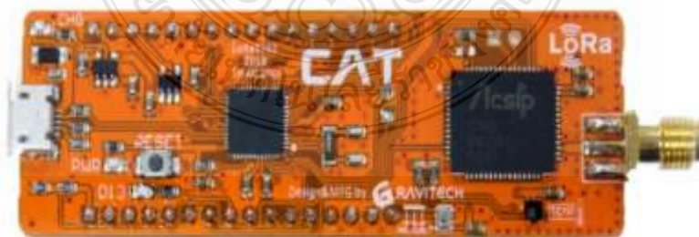
Figure 2.13 Board CAT Starter kit S767S [53]
