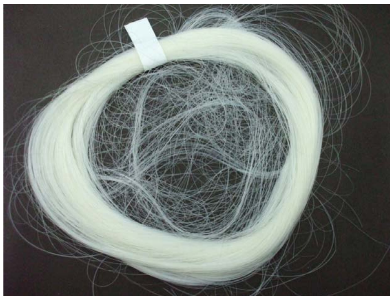
Fig. 9 Polypropylene/TiO 2 composite fibers for antibacterial applications.
