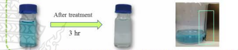
Fig. 4 Synthetic wastewater containing Methylene Blue: before and after treatment using the prepared microcapsules
