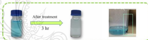
Fig. 2 Synthetic wastewater containing Methylene Blue: before and after treatment using the prepared microcapsules
