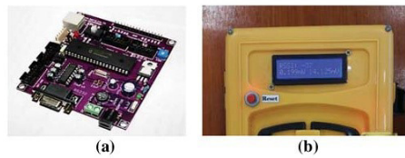
Figure 6: Rectenna power and voltage meter. (a) PIC16F877A microcontroller, (b) voltage multiplier circuit and LCD
