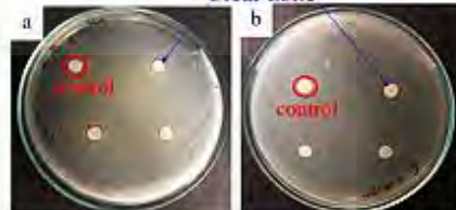
Antimicrobial test of polymer nanoparticle prepared by emulsion ITP (a) Staphylococcus aureus and (b) Zoonosis coli
