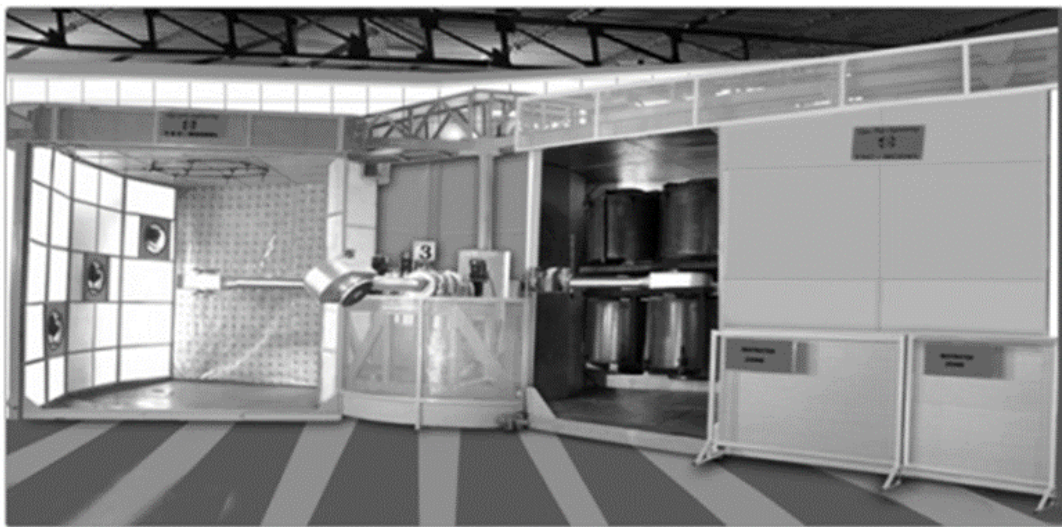
Figure 2.9 Fixed-arm type machine [1].
