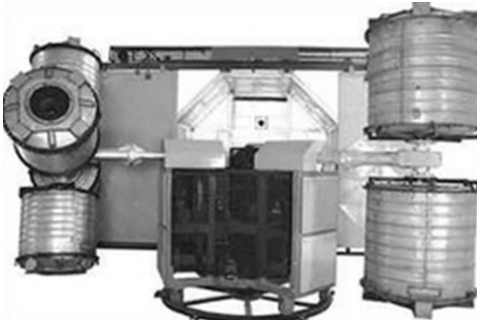
Figure 2.10 Independent arm type machine [1].
