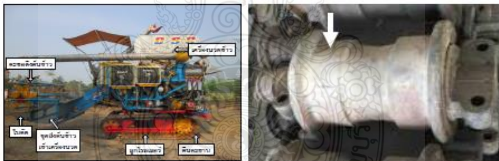
Figure 1 Combine harvesters And the wear position of the Roller (กิตติพงษ์, 2559)
