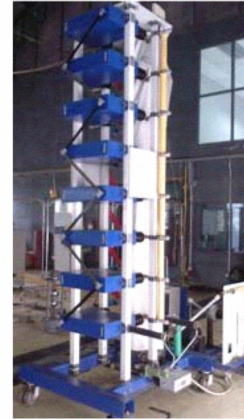
Fig.12: Lightning Impulse generator 800 kV
