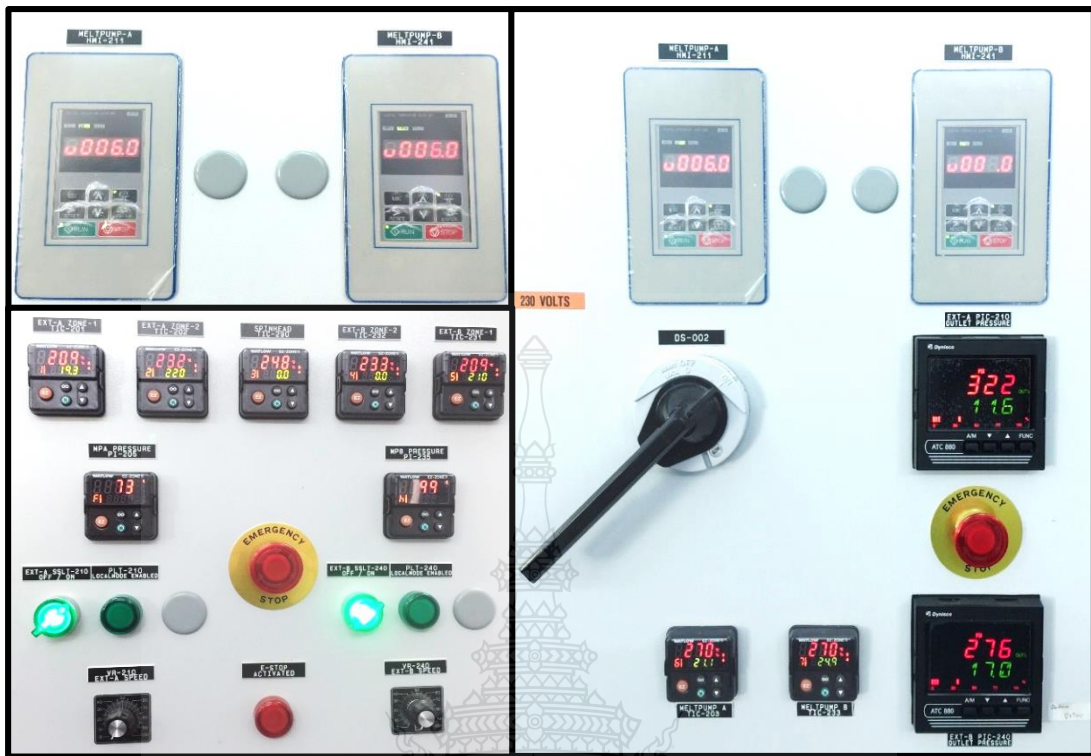
Figure 3.5 The condition control panel of The Hills' Lab Scale Bi-component Extruder Fed Spinning Machine Model LBS-100 in the experiments
