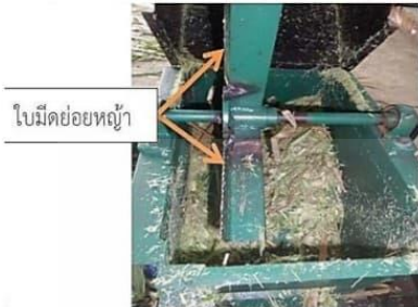
Figure 11 Closed up view of shredding unit.
