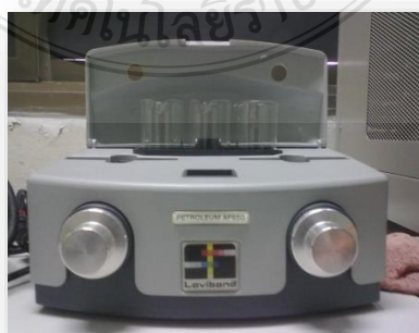
Figure 3.6 Color ASTM D 1500
