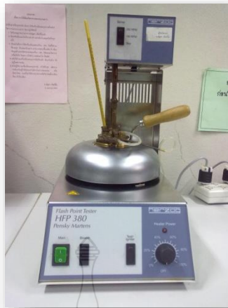
Figure 3.7 Flash point ASTM D 93
