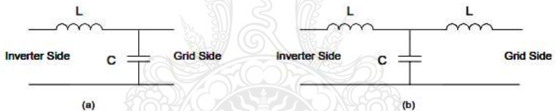
Figure 2.6 (a) A LC filter and (b) a LCL filter, as required for PV inverter harmonic filtering in line currents. [21]
