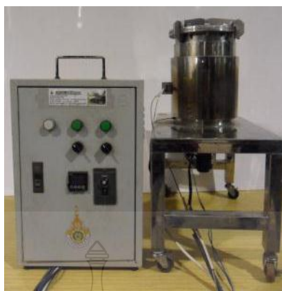
Figure 3.5 Thai made teflon-lined stainless steel autoclave and control unit.
