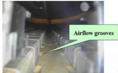
Fig.1 Airflow grooves on the stator slot.
