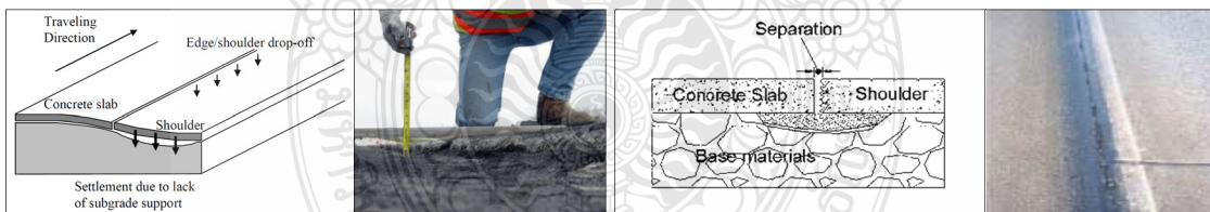
(I) Lane to Shoulder Drop Off
