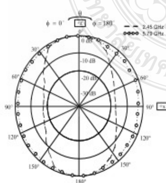
Fig. 10 radiation simulation at resonance frequency of 2.45 GHz and 5.79 GHz on x-y plane
