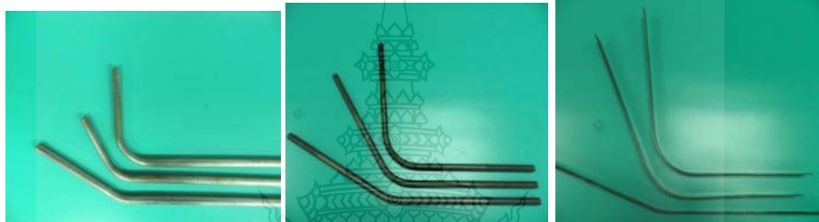
Figure 4 Workpiece of bending has been used 30, 60 and 90 degrees
