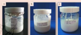
Fig. 5 Photos of PC emulsion prepared by the PIE technique in oil/water system using 2%wt PVA in oil at various SDS in continuous phase (%wt): a) 0.2; b) 0.5 and c) 1
