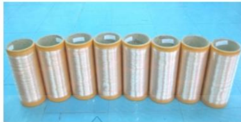
Fig 5. PLA:PBS blends fibers for melt spinning technique.
