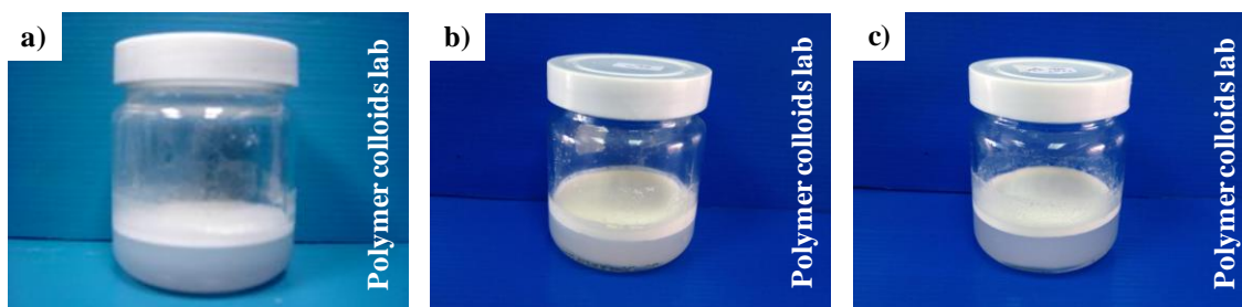
Figure 4.15 The suspension photos of P(DVB-MMA)/OD microcapsules prepared by microsuspension polymerization of DVB: MMA (wt %) (50:50) at various additional rates (mL/min): a) 2; b) 4 and c) 8
