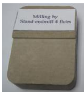
Fig. 6 The sample was milling by standard endmill 4 flutes
