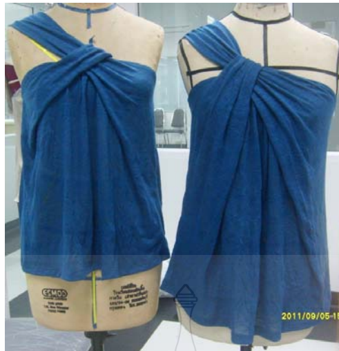
Figure 6: Comparison between the sampling made from the flat pattern making technique (left figure) and the draping technique (right figure)
