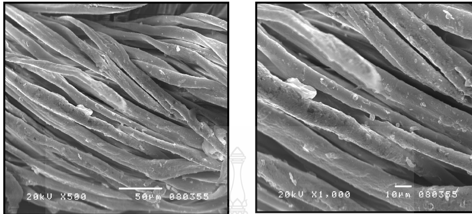
Figure 1 : Efficiency of the microcapsules coated onto the fabric using heat to dry.
