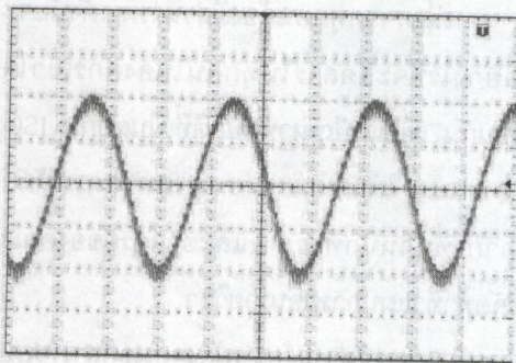
Fig.10. Output voltage waveform with resistive load. Horizontal scale: 5 ms/div; vertical scale: 0.2 V/div.
