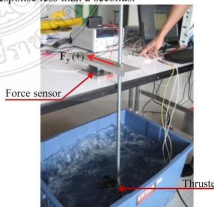
Fig.4 Experimental setup for thrust force measurement.
